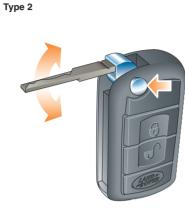
Key blade Press button (arrowed in illustration) to release the key blade.
